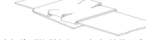
Sharp edged or misformed joints which do not appear as shown have to be taken away from the load immediately. The tensile strength of these joints is insufficient and they could cause serious injury. Having faulty joints proceed as follows:
