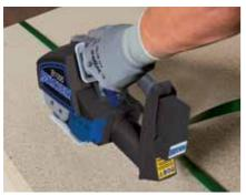
The B1000 can pull up to 1125lbs of tension and operate with both polypropylene and polyester plastic strapping, 5/8" to 3/4" wide, .031-.050" thick. No special change parts are
