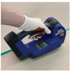
Uniquely designed to handle a wide range of applications. The B600 can pull up to 600lbs of tension. The B600 operates with polypropylene and polyester plastic strapping, (see specifications) 1/2" to 5/8" wide, .019 - .030 thick. The 14.8V Lithium Polymer (LiPo) battery weighs less
