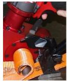
Press the trigger to pull the tension.
