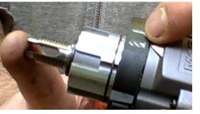
Remove drill selector ring and clutch plates.
