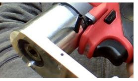
Install roll pin into 3/16" hole with a punch and hammer.
