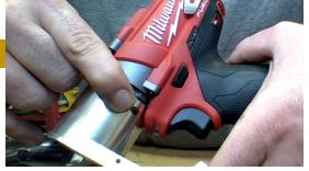
Slide drill into collar and clamp together.
