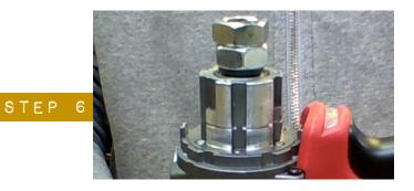
Grind drill shaft flush with the top of the nuts.
