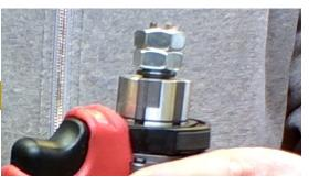
Attach two nuts on to drill shaft with red loctite.
