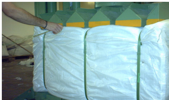
STRAPPING FIBER BALES USING PRESS SYSTEM
