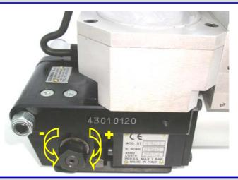
THE POLI MT CAN ALSO BE ORDERED WITH AN ADJUSTABLE CLUTCH SYSTEM CONFIGURATION - PARTICULARLY USEFUL TO HAVE UNIFORM TENSION ON STRAPS – IS NECESSARY INDICATE THIS OPTION ON THE ORDER
