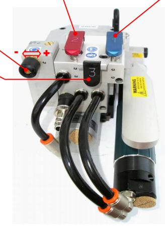
TURN THIS SCREW TO ADJUST THE GAP BETWEEN THE FEEDWHEEL AND LOCK STRAP PLATES
