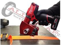
Squeeze handle, and pull the tool to the right to remove.
