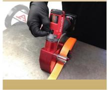
Select gear. Pull the trigger to desired tension.
