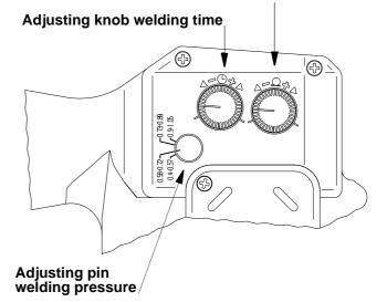
5.2.3 Adjusting the welding pressure
