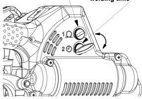
The adjustment knobs can be easily turned with a coin.
