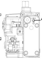
Adjusting screw welding time
