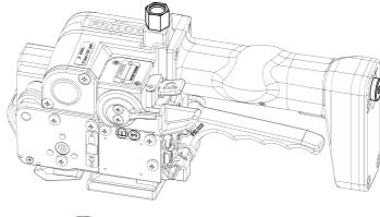
According to requirement the connection can also be assembled to the rear end of the tool.
