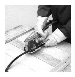
**4.** Using your right hand turn the ring of the turning valve **(a)** to the left, to the limit. The motor starts to run and tensions the strap. After reaching the desired strap tension release the ring. The turning valve closes automatically, the motor is stopped. (The strap tension is maintained by a free-wheeling mechanism.)
