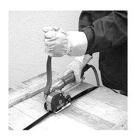
**6.** Bring cutting lever **(b)** back into its initial position and take hold of the cut off strap end with your left hand. Lift the compressed air motor **(f)** up to the limit and swing the tool to the right out of the strapping.
