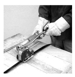
**5.** The right hand takes hold of the compressed air motor **(f)**, the left hand grasps the cutting lever **(b)** and pushes it rapidly forward up to the stop at the housing. Thus, the TITAN "no-seal-joint" is formed. At the same time the steel strap is cut off directly behind the joint.
