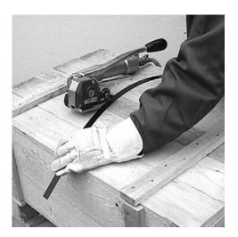
**2.** Pull strap end through until it is located in the middle of the packing unit below the upper strap and projects by a hand span.
