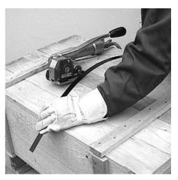
**3.** Hold both of the precisely overlapping straps firmly using your left hand. Using your right hand takes hold of the lifting lever **(c)** and cutting lever **(b)** and press together. Push both straps laterally along the housing wall into the tool as far as possible. A bit of the lower strap has to project out of the front of the tool. Release the levers **(c)** and **(b)**.
