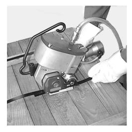
4. Use your right thumb to press the "tension strap"key button (a) until it engages the notch (g) (the compressed air motor Stops if the notch released) For PKE tools having built-in-free-wheeling mechanisms the "tension strap" key button (a) should be pressed until the desired strap tension has been achieved.
