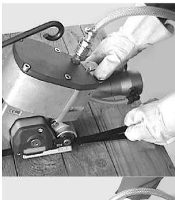
**6.** Take hold of strap end that is cut off with your left hand, press the air lever **(c)** and the compressed air motor **(f)** together using your right hand und swing the tool to the right out of the strapping.
