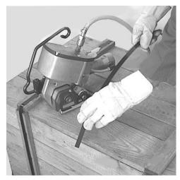
**2.** Pull strap end thought until it is located in the middle of the packing unit below the upper strap and projects a hand span.
